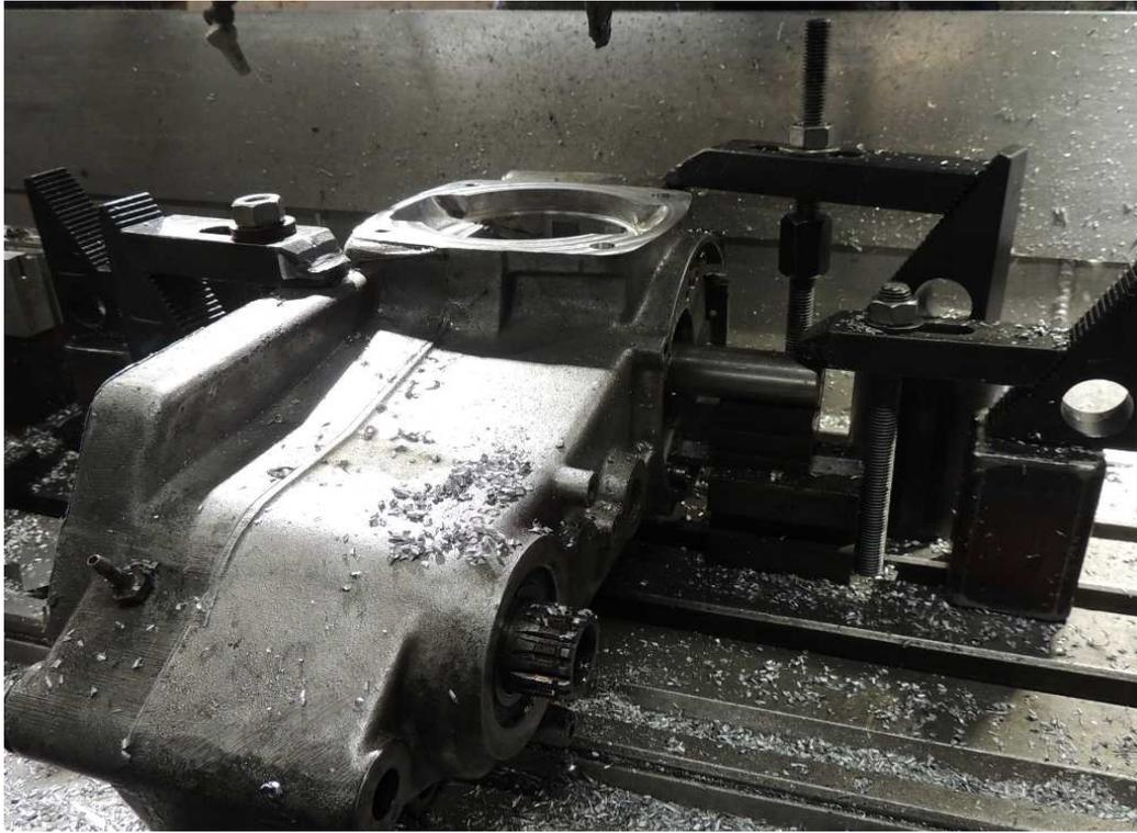
The next step is to rebuild the crank. The drive side shaft has worn oval, so it will be copper plated and the machined back to size. I have already built up the spline using TIG and a hard facing rod and hand ground it back to size. I TIGed quickly and only did one spline shoulder at a time to reduce the heat damage. The cranks are not hard at all, they are only 25 Rockwell C.
