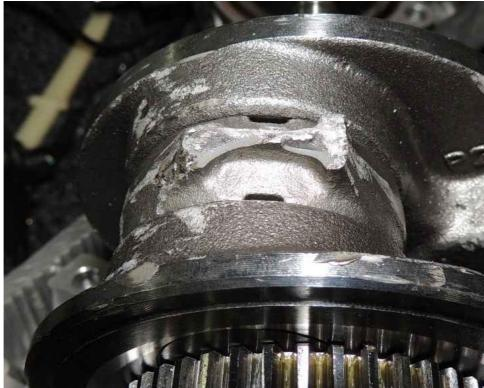
The rod has broke at the thick/strongest side near the base where there would be limited flex.
